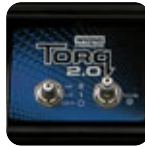
TBB145E COMMUTATORI HI/LO/OFF (ALTO/BASSO/STOP) E PULSE (IMPULSO) HI/LO/OFF AND PULSE TOGGLE SWITCHES
